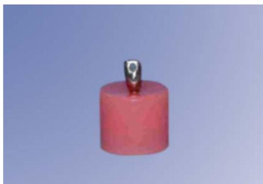
**Fig. 2:** Casted crown on the abutment
