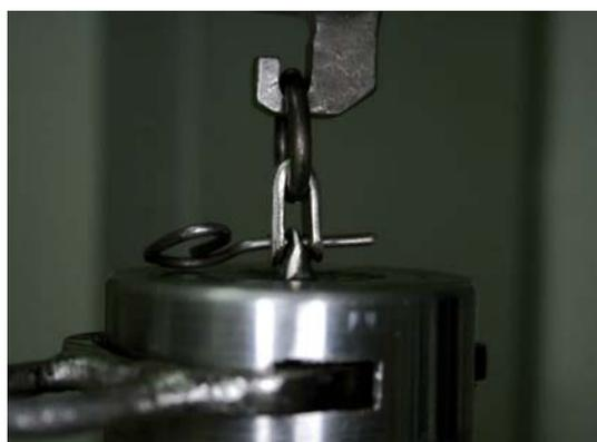
**Fig. 3:** Cemented crown on universal test machine before tensile test
