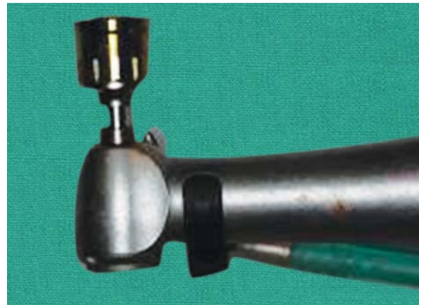
Fig. 4: Dome drill with 0.5 mm stopper placed on the surgical handpiece
